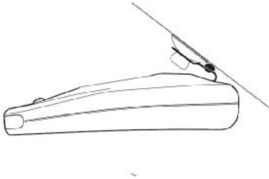
2 To adjust the **GPS & radar detector** on your windshield, use the Easy Mount adjustment button located on the top of the **GPS & radar detector**, and slide **GPS & radar detector** forward or backward to obtain a level horizontal position.
