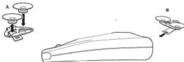
1 Depress the adjustment button on the top of the **GPS & radar detector** and slide the bracket into the slot until it is locked into the position which best fits the angle of your windshield (There are two options of installation available: Windshield mount or Dashboard mounting). For extremely horizontal or extremely sloped windshields, the bracket can also be bent to the correct angle.
