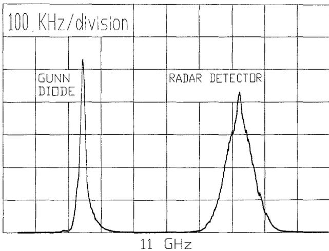
Figure 3. A comparison of the radar detector's VCO stability to that of a Gunn diode oscillator.
