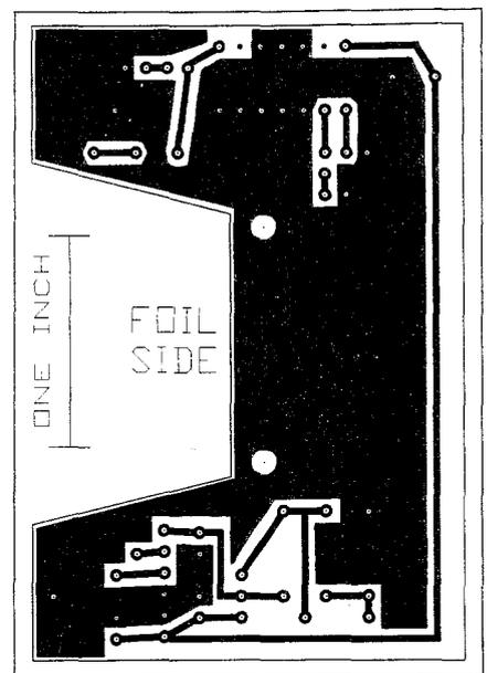
Figure 6. Foil side of the PCB.
