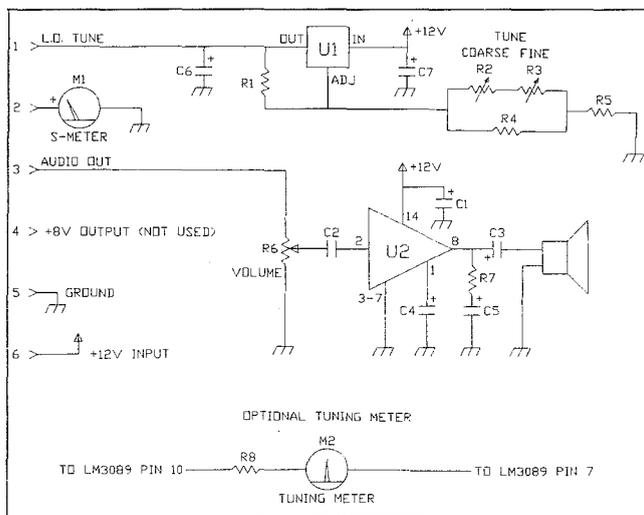
Figure 5. Schematic of the new circuit board.
